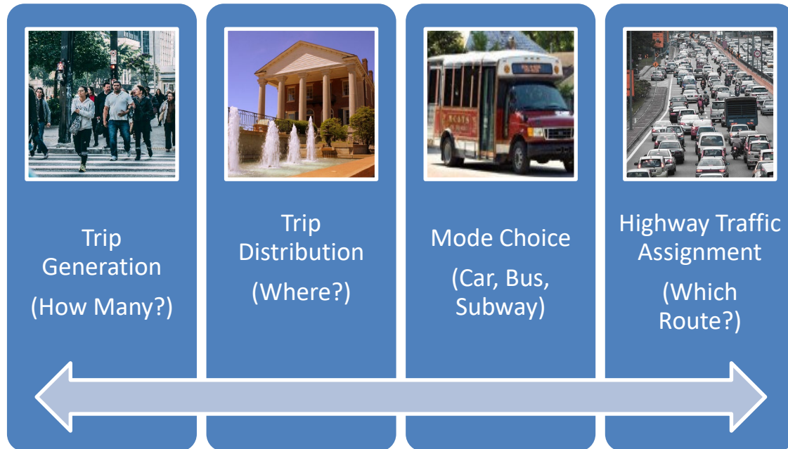
Figure 7 Four Step Travel Demand Modeling Process
