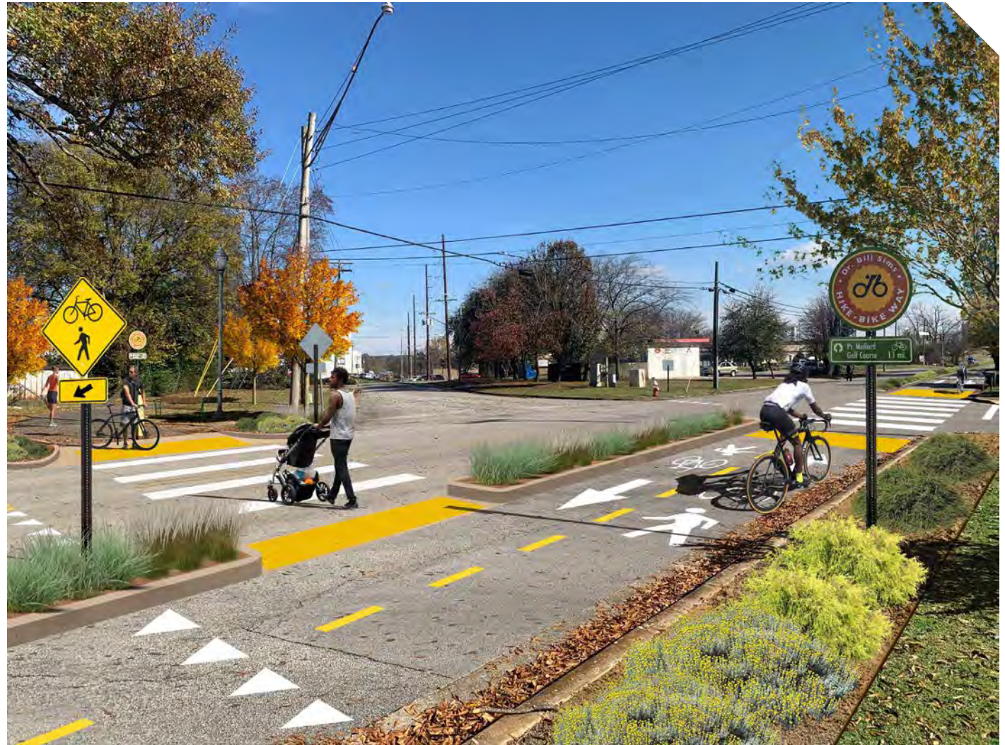
Proposed Separated Two-Way Cycle Track - Dr. Bill Sims Hike-Bike Way - Grant Street
